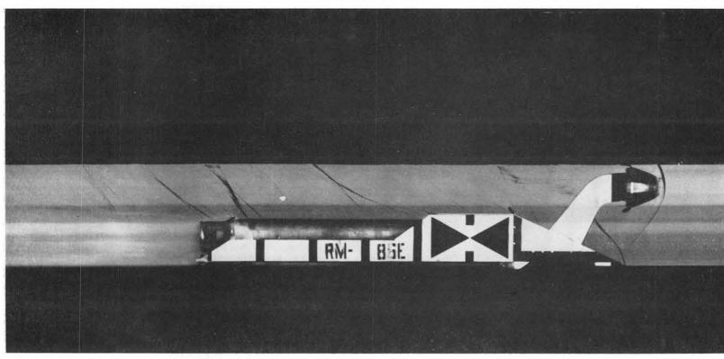
STREAKING PAST camera station at 1865 ft. per second, this thousand ft. of the run was through a man-made rainstorm. Black monorail rocket sled tests materials in the forward radome. Six lines are shock waves. Photography details in accompanying article.
